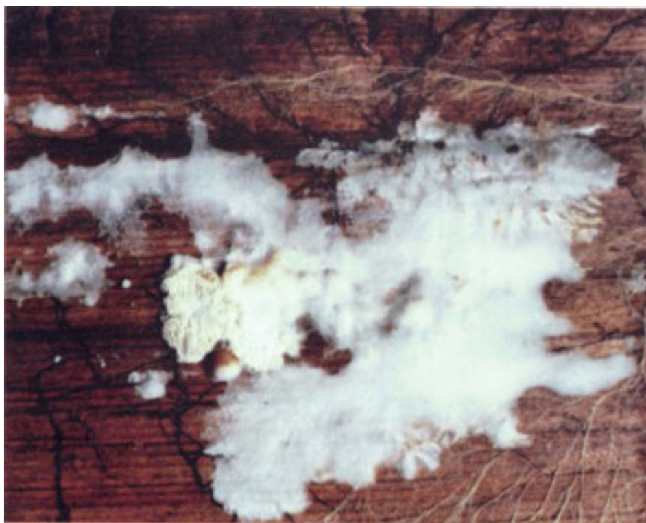
Early dense white vegetative growth of one fungus, late cream/fawn vegetative growth of a second fungus, dark brown/black water-conducting strands of a third fungus. Off centre can be seen the pored surface of a young reproductive fruit body.
