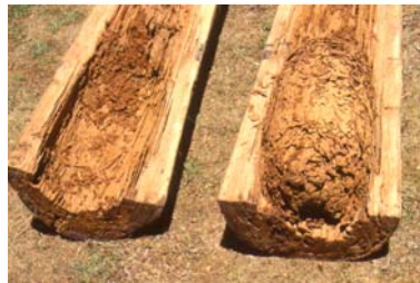
(b) Termite nest in a timber post
